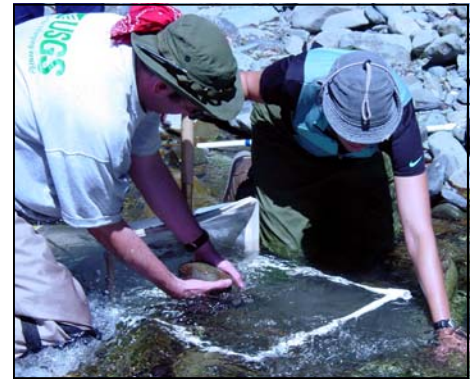
Researchers using a Slack sampler, which standardizes the area of sediment and water where insects are found
