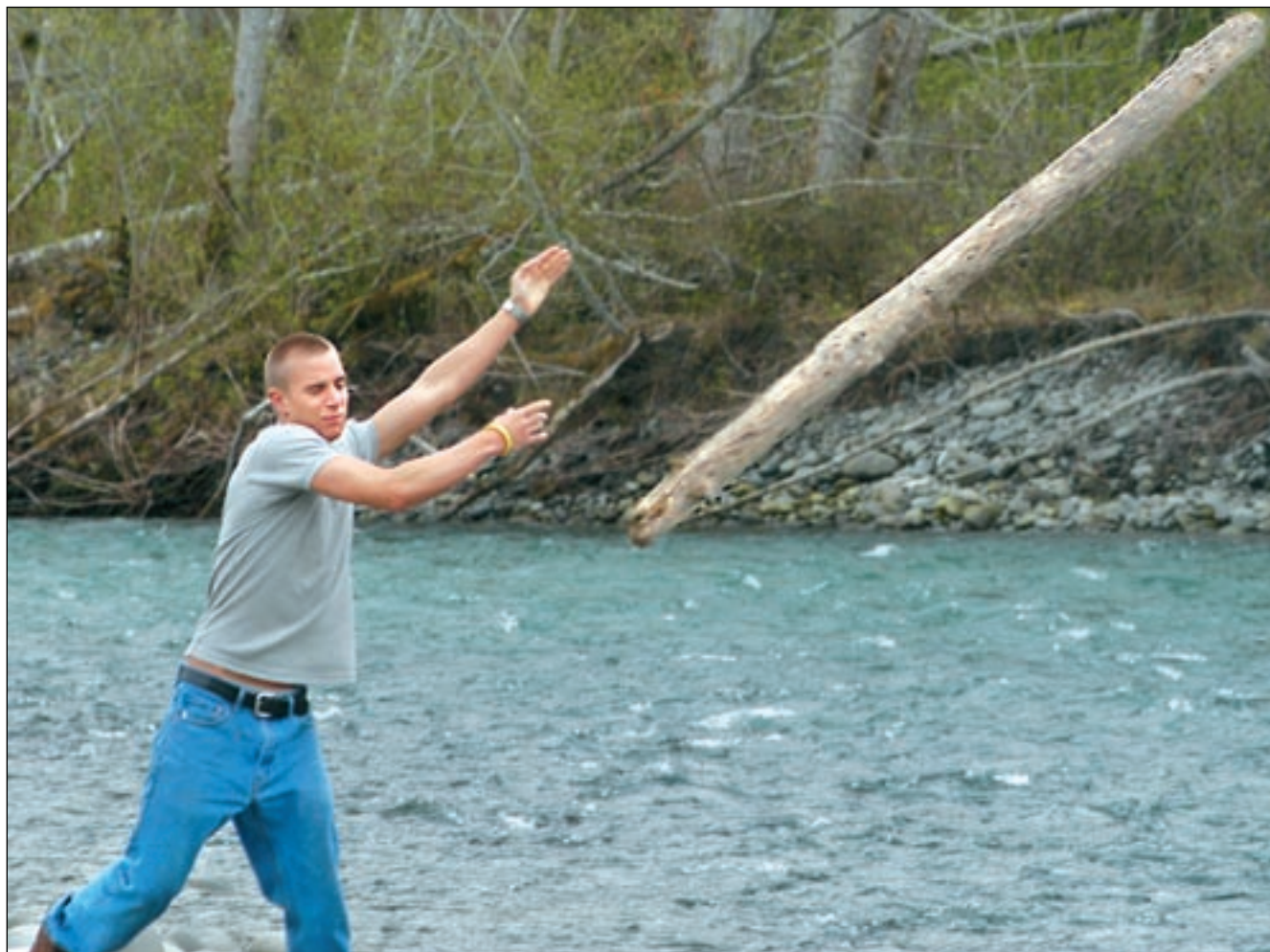
Logan Mead heaves a log into the Elwha River so observers in his team can time the float over a measured course to determine the speed of water in the river.
